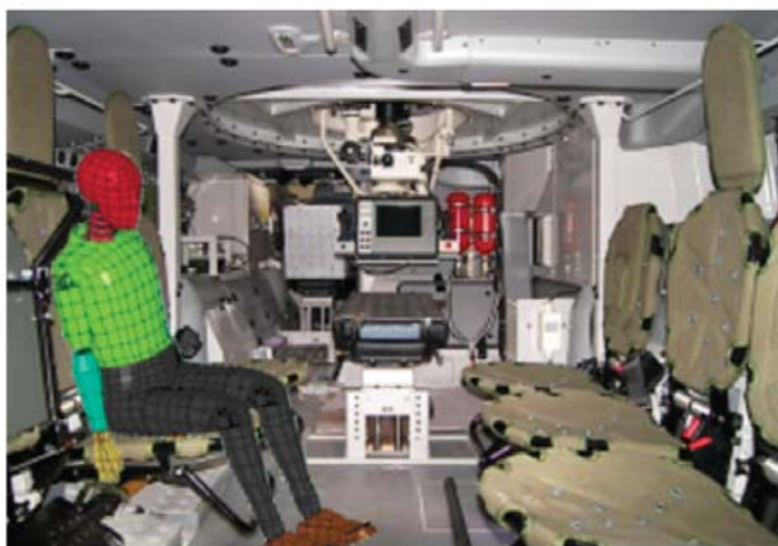
Fig. 7a) - Interior of the crew compartment of the armored personnel carrier, b) - Hybrid III dummy model
